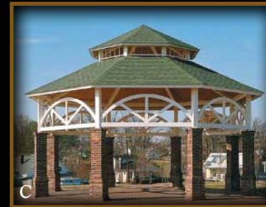
C Cannon Park, Salisbury, NC: This 30' custom model has a 2" x 6" T & G subroof with fiberglass shingles, a raised 2nd tier, custom curved ornamentation and brick columns, giving a feeling of Southern hospitality. No field welding required!
